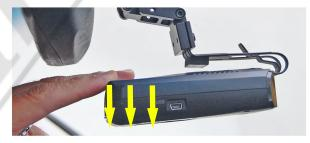
**STEP 3** - If the RD is too close to the bottom of the mirror, You may access the buttons on top of the RD by gently pushing downward on the front of the RD with one finger and push the desired button with another finger. Then allow the RD to return to it's original position by gently letting it spring upward. When accessing the buttons, be sure to push the RD downward just enough for your finger to fit between the RD and mirror. **Do not push down more than what is needed.**
